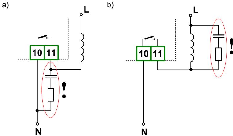
Figure 4.9. Examples of suppression circuit connection:
