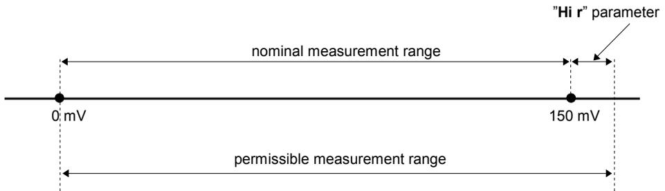
Figure 6.1. Definitions of measurement ranges in mode 0 ÷ 150mV
