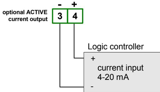
Figure 4.12. Example of current outputs connection
